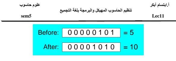
If binary 00001010 (decimal 10) is shifted left by two bits, the result is the same as multiplying 10 by 2<sup>2</sup>
