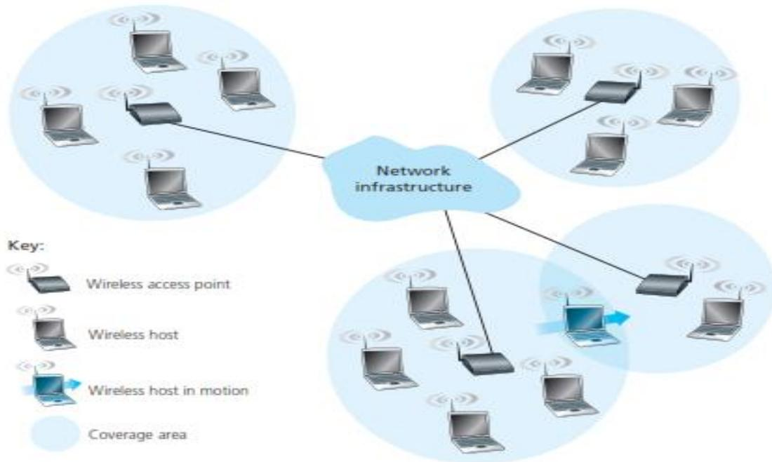
**Figure 6.1** ♦ Elements of a wireless network
