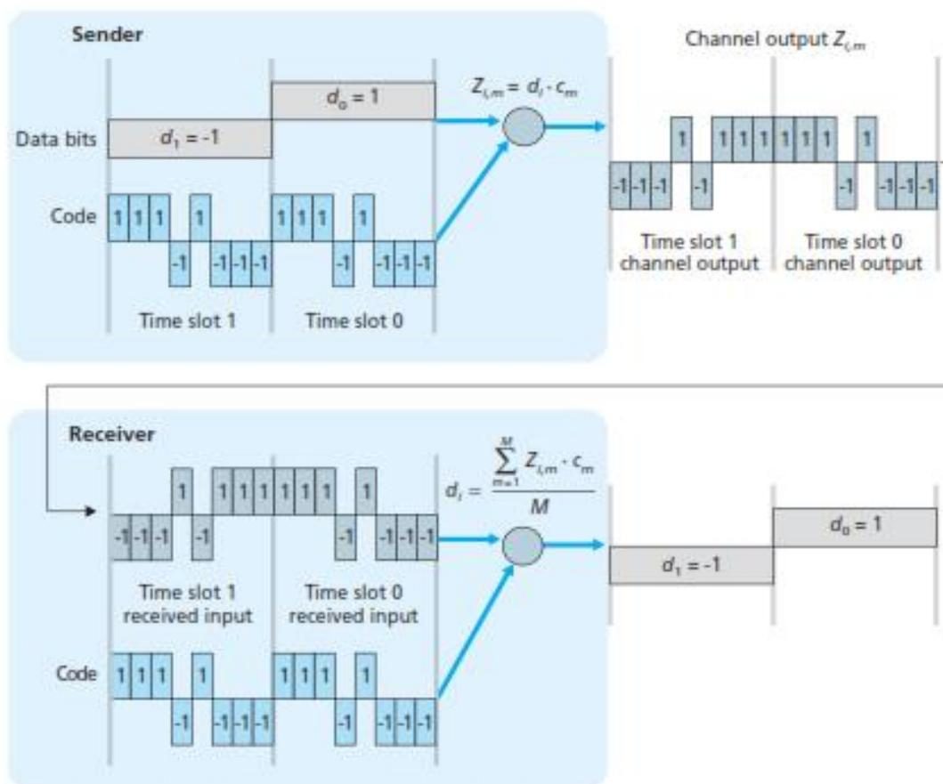
**Figure 6.5** • A simple CDMA example: sender encoding, receiver decoding
